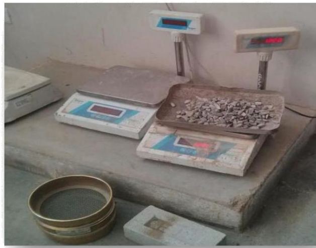
Figure 2: Weighing of Aggregate
