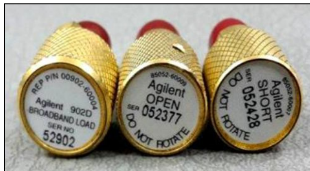
Figure 6. Calibration Kits for Reflection Measurement using PNA
