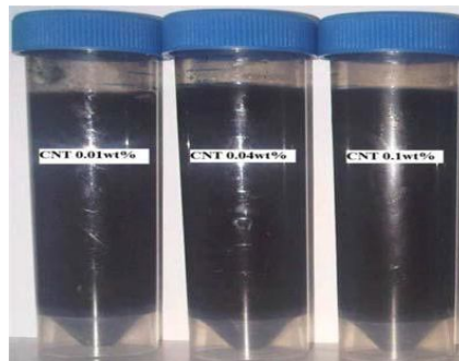
Fig. 1. Stable CNT Nanofluids after 10 min Homogenization and 4 hr Sonication
