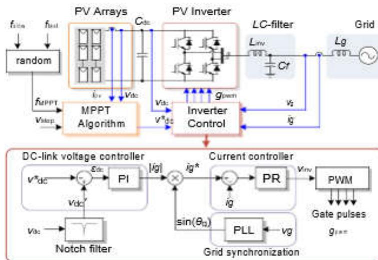
Fig. 1. System diagram and control structure of single-stage single-phase PV inverter (PI - Proportional Integral, PR - Proportional Resonant, PWM - Pulse Width Modulation, PLL - Phase-Locked Loop).
