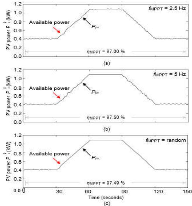
Fig. 7. Measured PV power extraction of the PV inverter under the trapezoidal solar irradiance condition with the MPPT sampling rate of: (a)  $f_{MPPT} = 2.5$  Hz, (b)  $f_{MPPT} = 5$  Hz, and (c)  $f_{MPPT} = \text{random}$ .
