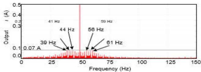
Fig. 6. Frequency spectrum of the output current  $i_g$  of the PV inverter operated at 10 % of the rated power (i.e., 0.3 kW) with randomly applied MPPT sampling rate of  $f_{slow} = 2.5$  Hz and  $f_{fast} = 5$  Hz.
