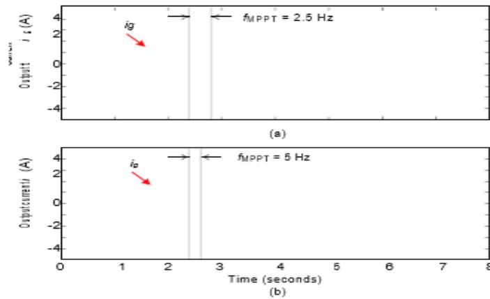
Fig. 3. Experimental waveforms of the output current  $i_g$  of the PV inverter operated at 10 % of the rated power (i.e., 0.3 kW) with the MPPT sampling rate of: (a)  $f_{MPPT} = 2.5$  Hz and (b)  $f_{MPPT} = 5$  Hz.
