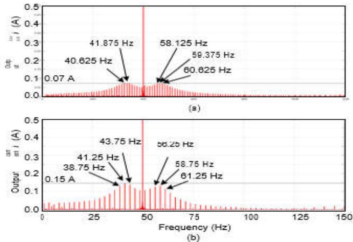
Fig. 4. Frequency spectrum of the output current  $i_g$  of the PV inverter operated at 10 % of the rated power (i.e., 0.3 kW) with the MPPT sampling rate of: (a)  $f_{MPPT} = 2.5$  Hz and (b)  $f_{MPPT} = 5$  Hz.
