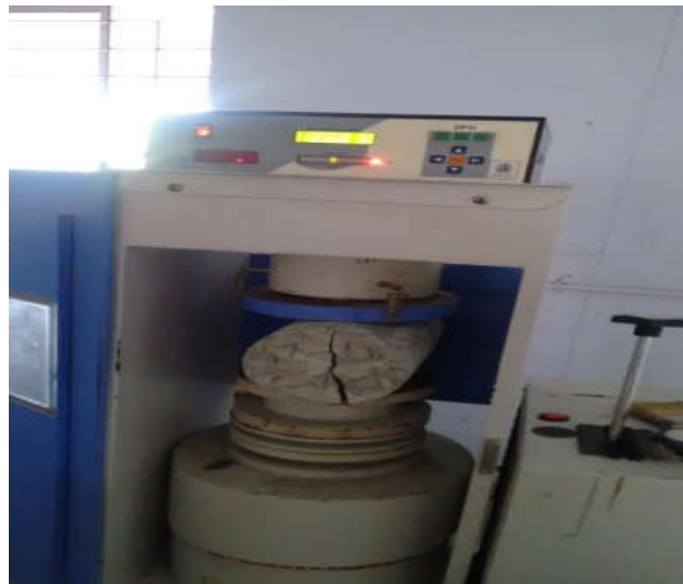
Figure 4 Split Tensile Strength Test
