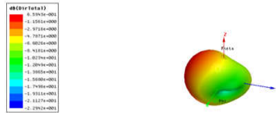
Figure 3.4.1 Simulation result of directivity
