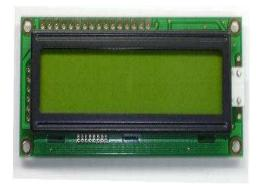
In this project 16\*2 LCD is used to display message. It is basically used for displaying purpose on the occurrence of accident it would display the accident detected message
