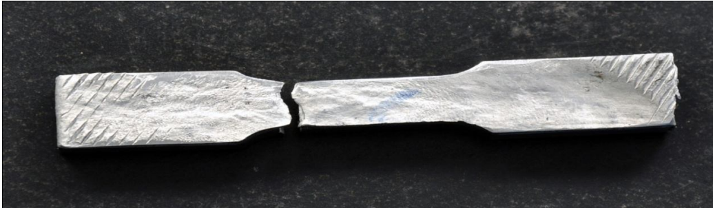
Figure 4. Fractured Specimen after tensile test
